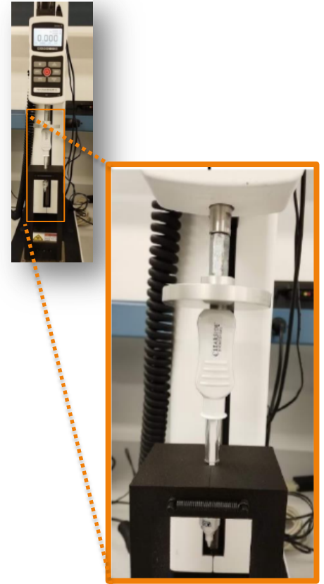
Test Set-Up: Syringe Glide and Break Force
